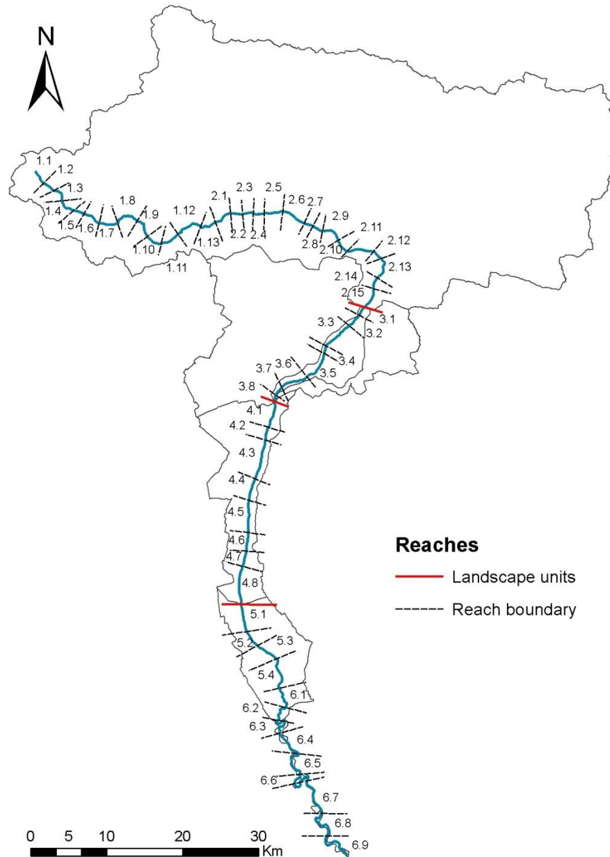
Figure 2.3 The Tagliamento River was delineated into 57 reaches. Reach divisions align first with the landscape unit and segment divisions, and are then delineated based on channel planform, presence of tributary confluences, changes in channel slope and/or width.
