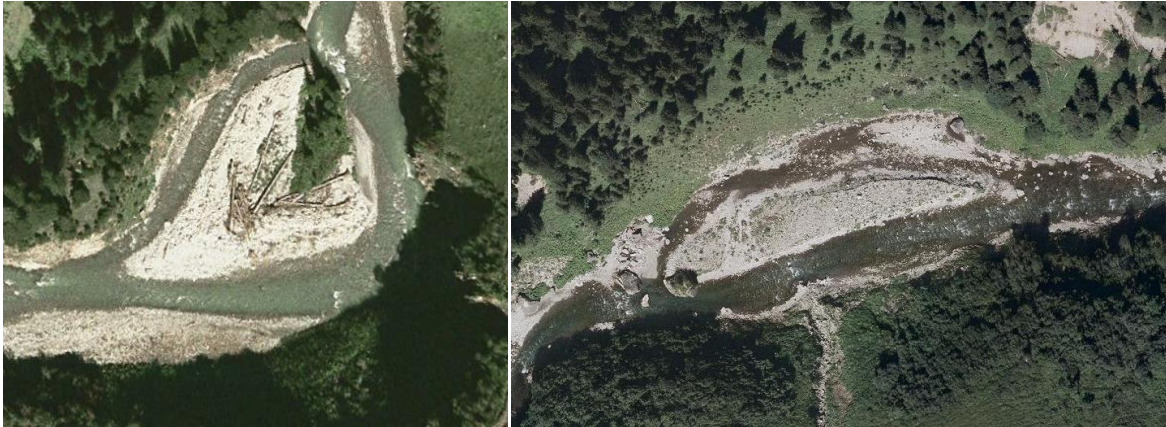
Figure 4.37 Small braiding sections with (left) and without (right) vegetation on the bars (VoGIS, 2013).
